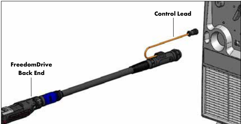
Fig. 10 Connecting the FreedomDrive Control Lead
