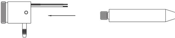
2. If required for your particular feeder, slip the power lug over the adapter plug. Do not tighten, as you will need to locate the correct position once installed on the feeder.
