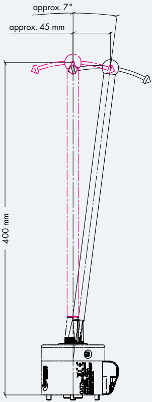
Figure 4: Maximum deflection in X- and Y-axis
