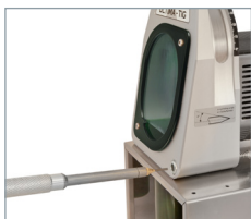
Precise adjustment of the electrode's stick-out.
